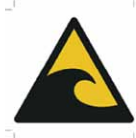
Figure 4.9 Signage used to indicate "Tsunami hazard zone".
